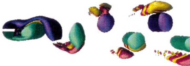
FIGURE 4. View of the alternating and streamwise vortex structures topology in the near wake. Iso-vorticity surfaces  $\omega_x = \omega_z = 0.25$ .
